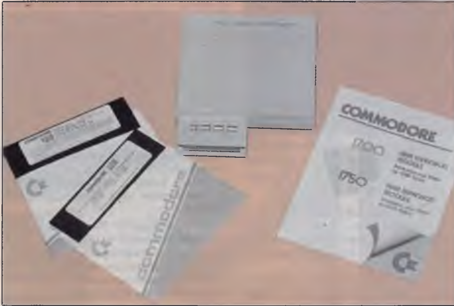
Figure 1. The 1700 and 1750 are RAM expansion units for the 128 and are one of Commodore's better kept secrets. They are identically sized cartridges which plug into the expansion port. The only difference between them is the amount of memory they offer – the 1700 provides an additional 128 Kbyte, while the 1750 provides a massive 512 Kbyte.
