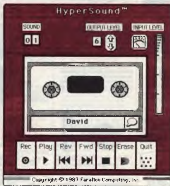
The HyperSound control panel for the MacRecorder. HyperSound is specifically designed to add sound to HyperCard.
